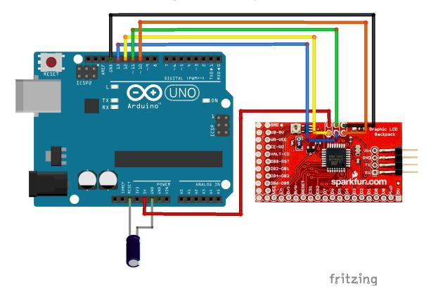
Figure 15: Arduino connections for ISP programming
