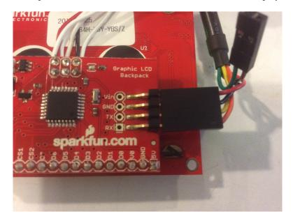
Figure 10: Serial Connection
