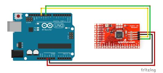
Figure 12: Arduino connection using software serial
