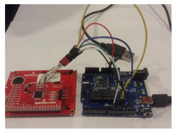
Figure 16: Backpack Programming from an Arduino
