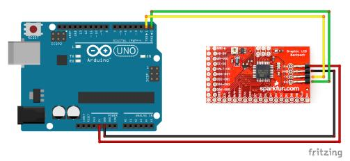
Figure 11: Arduino connection using hardware serial
